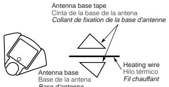
Cut the attachment tape to leave a space in between for the heating wire. Attach the tape to the antenna base section and then stick onto the glass surface.
