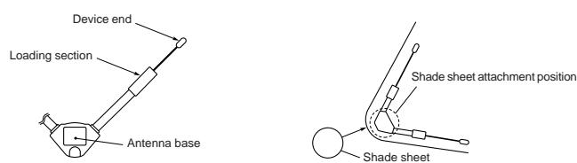
**Note:** The shade sheet is used to hide the antenna base from the glass exterior.
