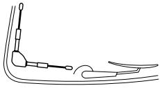
Move the antenna's attachment position upwards to avoid interference.
