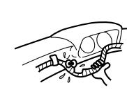
Secure together with the vehicle's wire harness or using a clamp.
