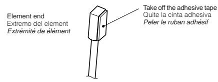
Take off the adhesive tape from the device end.
