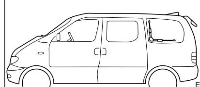
Attach to the inside of the rear, side windows on either side.
