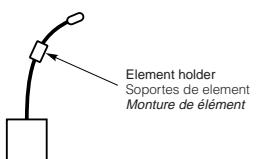
Secure the bent portion with the element holder.
